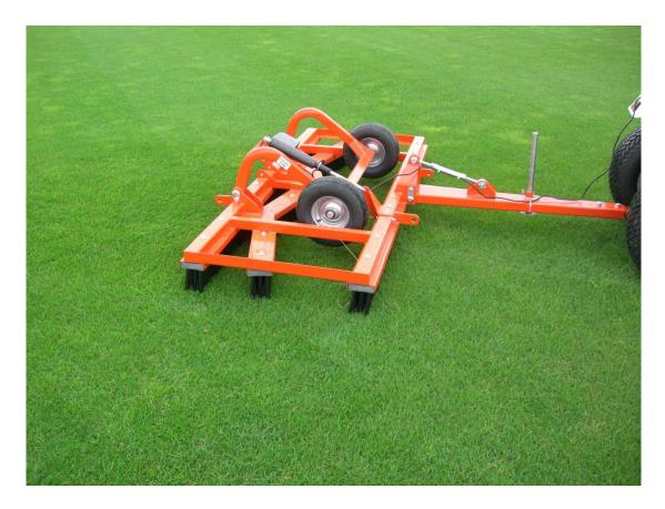
**Technical data** 3pt linkage trailed Length in m 1.005 2.09 Working width in m 1.87 1.87 Weight 110 kg 90 kg Mounting rear-3-pt hitch cat 1 towbar Drive ground-driven ground driven Lifting electric
